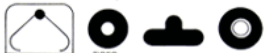
DIE CUT BUTTON SLOT FIBER-REINFORCED PATCH BUTTON SLOT PATCH WITH METAL EYELET
