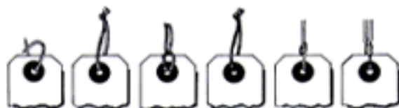
OVAL DEADLOCK KNOTTED STRING LOOPED STRING KNOTTED ELASTIC SINGLE WIRE DOUBLE WIRE
